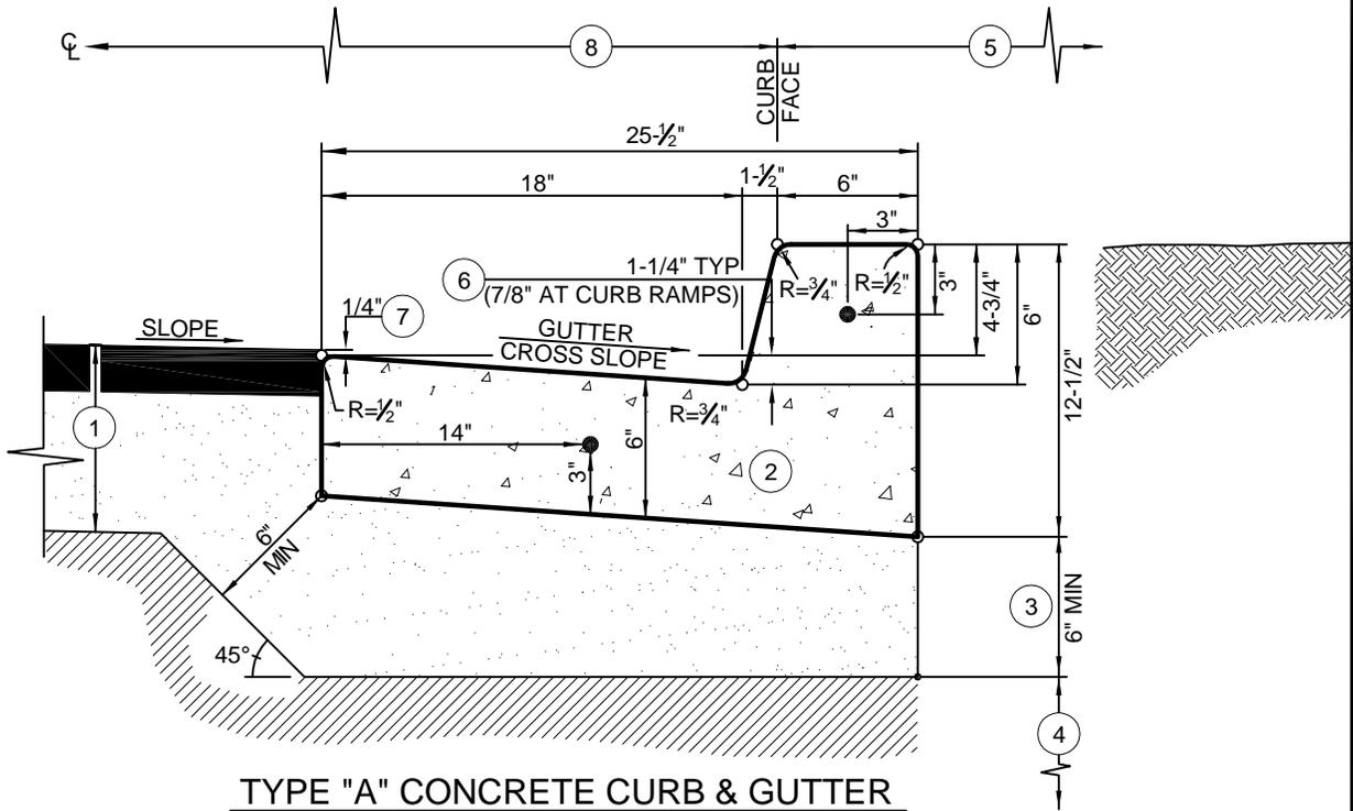
**TYPE "A" CONCRETE CURB & GUTTER**
