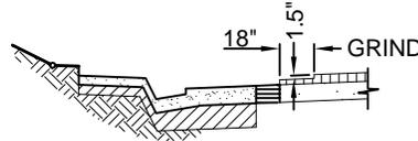
STEP 5: WHEN EXISTING AC IS P 3.5" THICK, GRIND 18" WIDE x 1.5" DEEP OF OFF EXISTING ASPHALT SURFACE.
