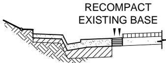
STEP 4: RECOMPACT EXISTING BASE SECTION TO 95% RELATIVE COMPACTION.
