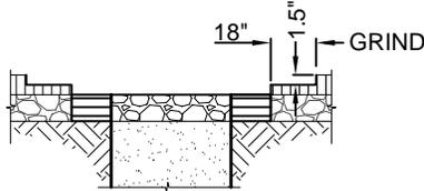
STEP 5: WHEN EXISTING AC IS P3.5" THICK, GRIND 18" WIDE x 1.5" DEEP OF OFF EXISTING ASPHALT SURFACE.
