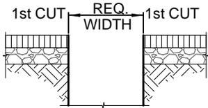
STEP 1: SAWCUT PER TO CONSTRUCT TRENCH PER U-4. SAWCUT SHALL FOLLOW ALIGNMENT OF STRUCTURE
