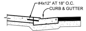
WHEN CURB & GUTTER IS PLACED PRIOR TO DRIVEWAY CONSTRUCTION THEN THE NEW DRIVEWAY SHALL BE DOWELED INTO THE CURB AND GUTTER WITH #4x12" AT 18" OC
