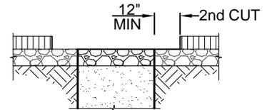
STEP 3: SAWCUT PER NOTE 1 TO REMOVE AN ADDITIONAL 12" MIN OF ASPHALT SURFACE.
