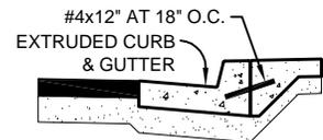
WHEN EXTRUDED CURB & GUTTER IS USED EXTRUDING MACHINE MUST BE CAPABLE OF PLACING A DENSE GRADE OF CONCRETE. SIDEWALK PORTION MUST BE PLACE WITHIN 1 HOUR OF EXTRUDED CURB & GUTTER UNLESS OPTIONAL JOINT IS USED.
