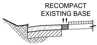
STEP 4: RECOMPACT EXISTING BASE SECTION TO 95% RELATIVE COMPACTION.
