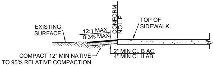
**SECTION A-A: ASPHALT CONCRETE RAMP**
