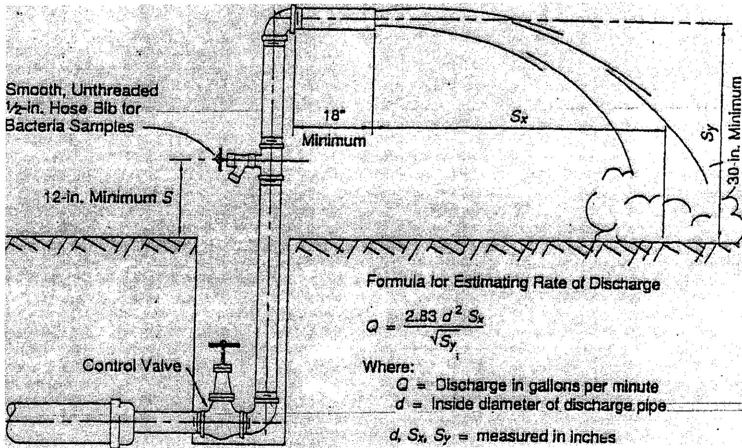
NOTE: This figure applies to pipes up to and including 8-in. (200 mm) diameter.
