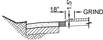
STEP 5: WHEN EXISTING AC IS P 3.5" THICK, GRIND 18" WIDE x 1.5" DEEP OF OFF EXISTING ASPHALT SURFACE.
