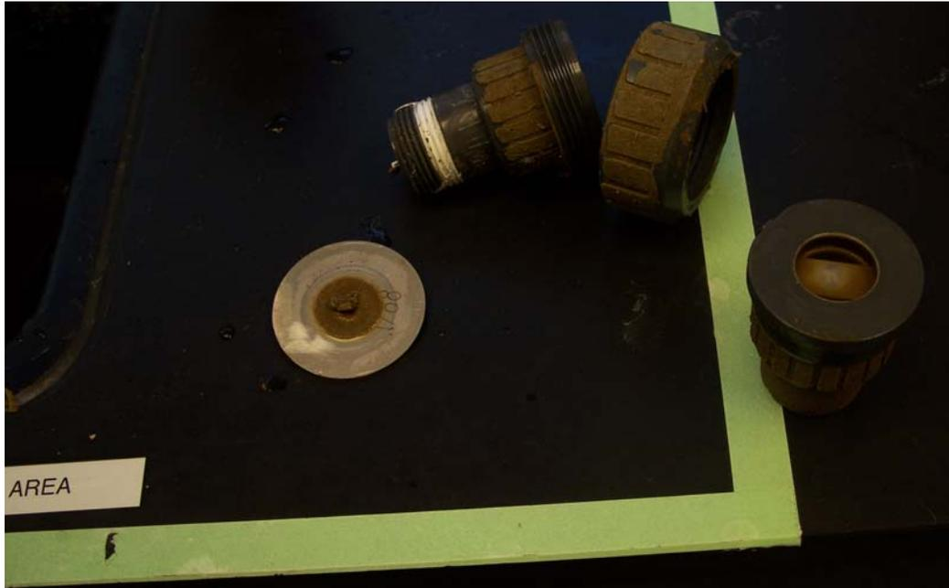
Photo 1: Scale formation plugging the DAF diffuser nozzles
