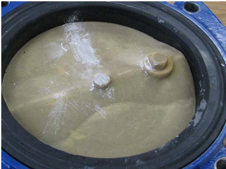
Photo 2: Excessively thick scale layer on the metal surface of a butterfly valve.
